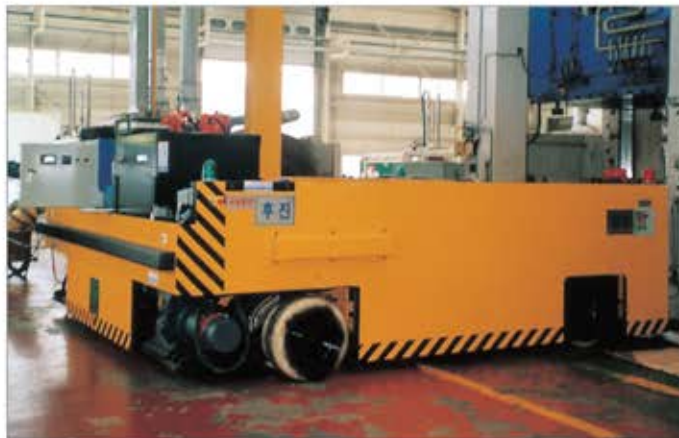
▲ MANUFACTURED AND DELIVERED TO BUGANG FACTORY OF HANWHA CHEMICAL-20TON CAPACITY OF TRACKLESS ELECTRIC TRANSPORTER CAR ▲ EASY IN AND OUT OF MOLD IN PRESS MACHINE BY ATTACHING ENTRY/EXIT DEVICE OF MOLD AND HEIGHT ADJUSTMENT DEVICE
