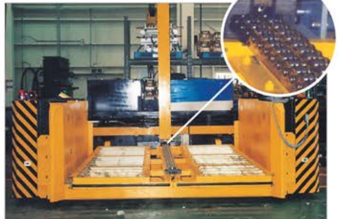
▲ MANUFACTURED AND DELIVERED TO BUGANG FACTORY OF HANWHA CHEMICAL-20TON CAPACITY OF TRACKLESS ELECTRIC TRANSPORTER CAR ▲ EASY IN AND OUT OF MOLD IN PRESS MACHINE BY ATTACHING ENTRY/EXIT DEVICE OF MOLD AND HEIGHT ADJUSTMENT DEVICE
